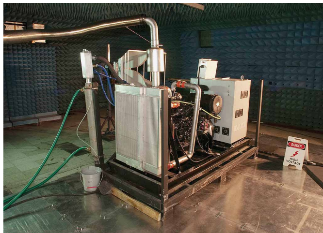
FIGURE 6. Chambers designed for MIL-STD-461 compliance tests don’t need turntables; cables for these tests can run on the chamber floor. Courtesy of Dayton T. Brown.
