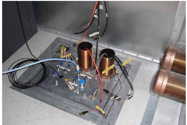
FIGURE 5. A floor-mounted panel provides power and signal cables with access to the inside of a chamber. Courtesy of Intertek.
